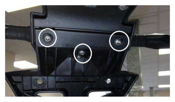
2. Remove the 5 bolts (M6 x 14mm) and 4 screws securing the under-tray to the machine and remove.
