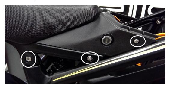
5. Remove the seat under panel by removing the 4 screws securing it to the unit. Note; this is necessary to be able to remove the seat from the assembly.
