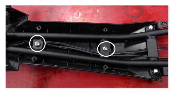
8. Turn the unit over and remove the 2 bolts (M6 x 14mm) securing the panel to the subframe and separate the pieces.
